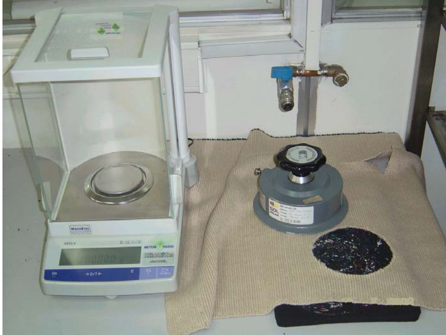
Fig. 5.5 Sample cutter and balance to determine fabric mass ( \text{g/m}^2 )
