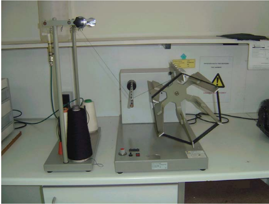
Fig.5.1 Apparatus for measuring the length of the skein
