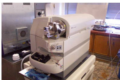
Figure 7. Picture of the instrument in the laboratory ( left ) and schematic presentation of the Q-TRAP ( right ).
