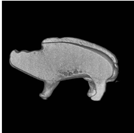
Fig. 5.2: Neutron Tomography: a virtual section through the wild boar from Windisch-Vindonissa, AG (Kantonsarchäologie Aargau). You can see some casting defects in the massive matrix.
