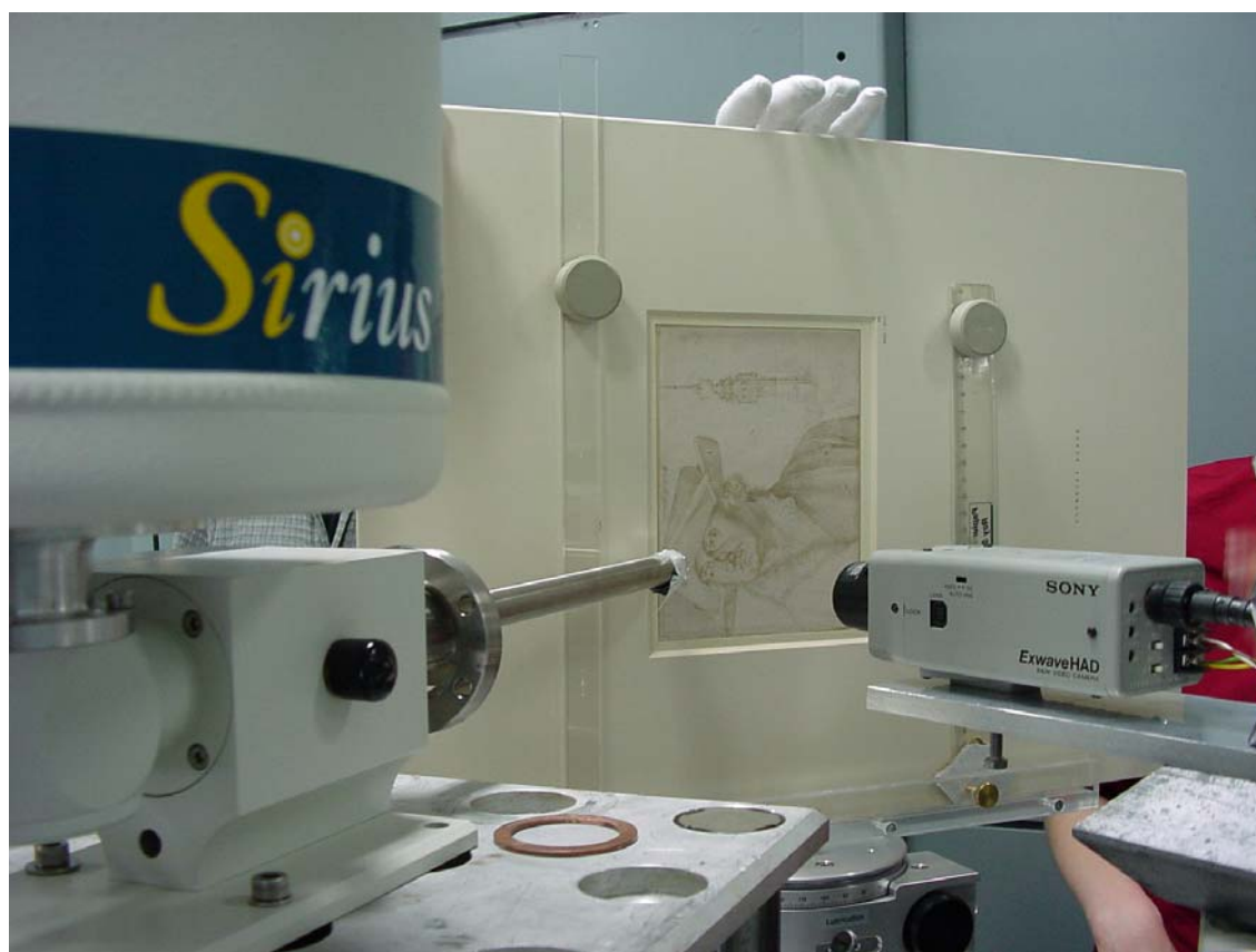
Fig. 1: Silverpoint drawing of the Netherlands sketch book by Albrecht Dürer 'Lazarus Ravensburger and the tower of Lier' (Berlin KdZ 35r, 13.0x17.0 cm, 1520) in front of the BAMline at BESSY with Si(Li) detector equipped with an aluminium filter and a video camera for sample positioning.
