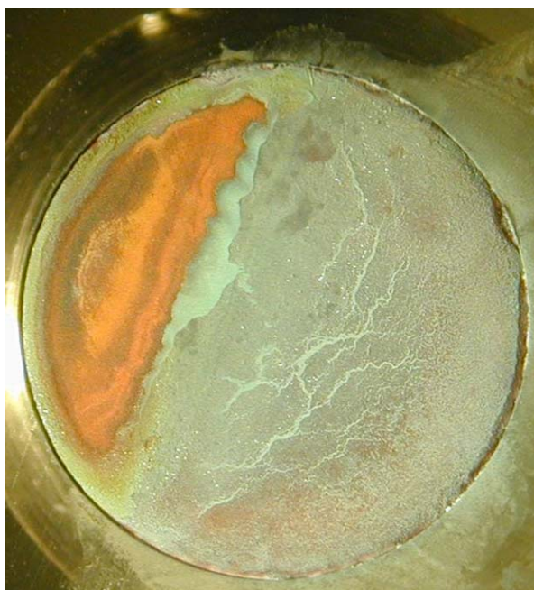
Fig. 11: Corroded copper electrode. The corrosion product is mostly nantokite.
