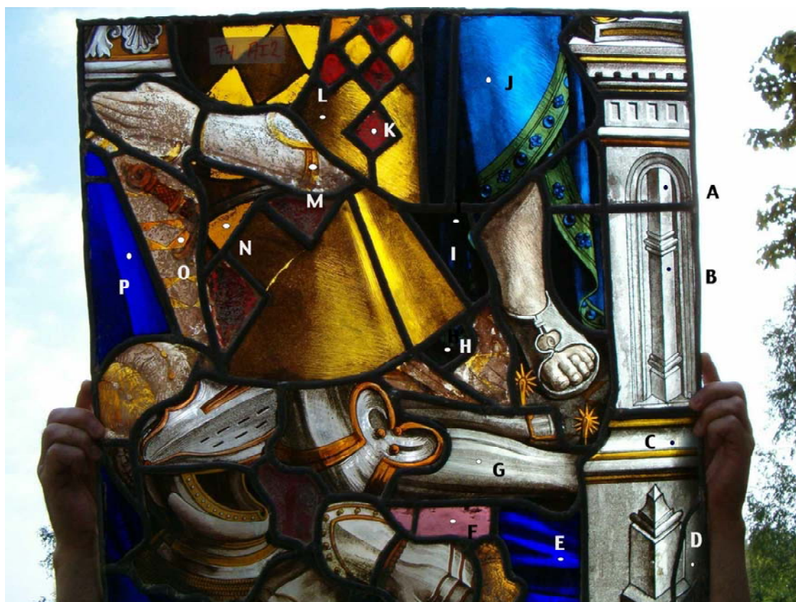
Fig. 2: View of the stained glass panel with the proton impact spots.
