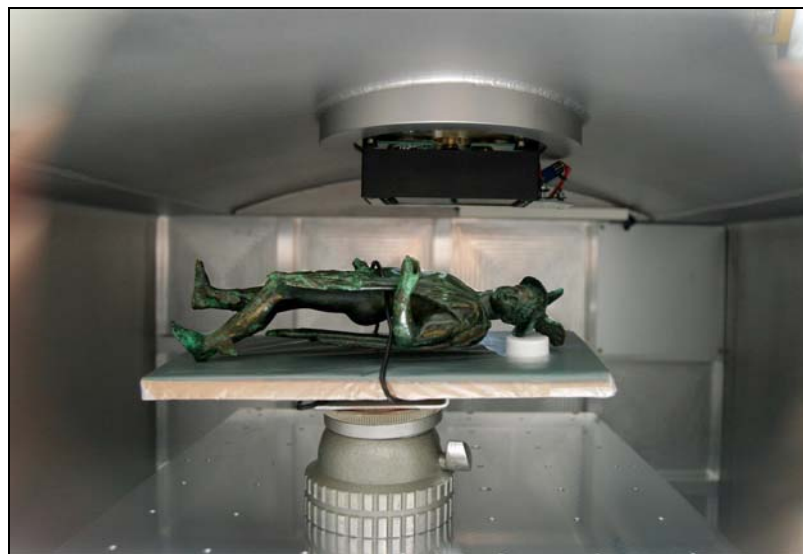
Fig. 6: One museum object in the measurement position inside the XRF chamber in the laboratory of the Swiss National Museum.
