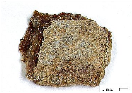
Fig. 1: Heavily corroded original fragment from London: overview.
