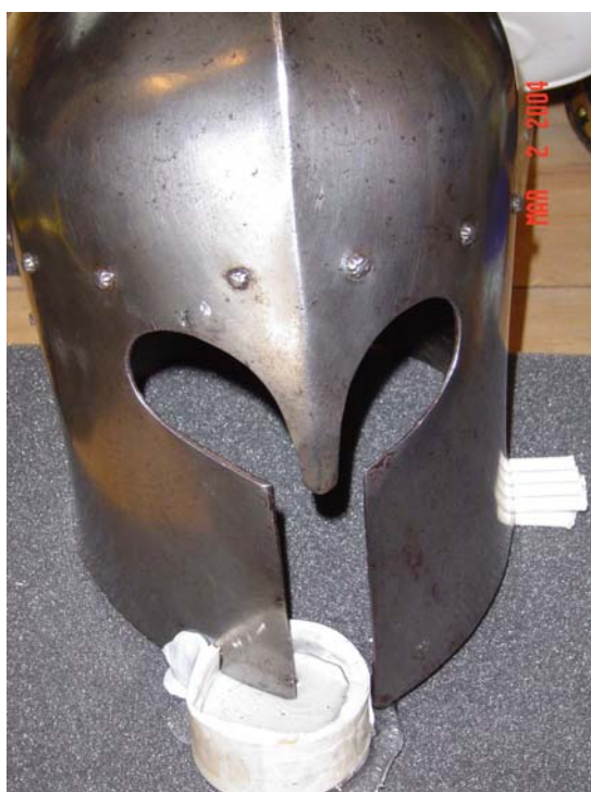
Fig. 1: Polyester resin curing around the edge of a 15 th century helmet (barbute) from the Wallace Collection (Inventory No. A75).
