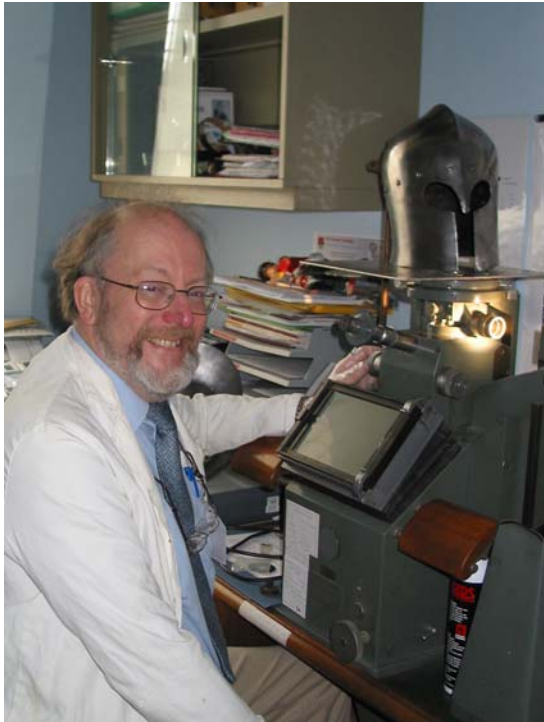
Fig. 3: Inverted microscope set-up. Examining the microstructure of the 15 th century barbuta.
