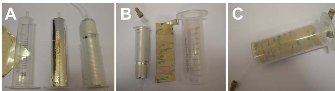
Figure 5 | (A) reflective tape around a 20 mL syringe, followed by the PFA microtubing coiled around
