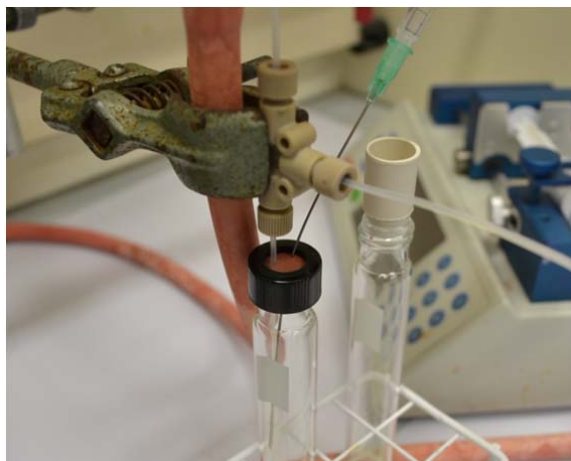
Figure 10 | Example of a reactor exit and reaction mixture collection. A PEEK tee micromixer is used to dilute or quench the reaction stream exiting the photomicroreactor.
