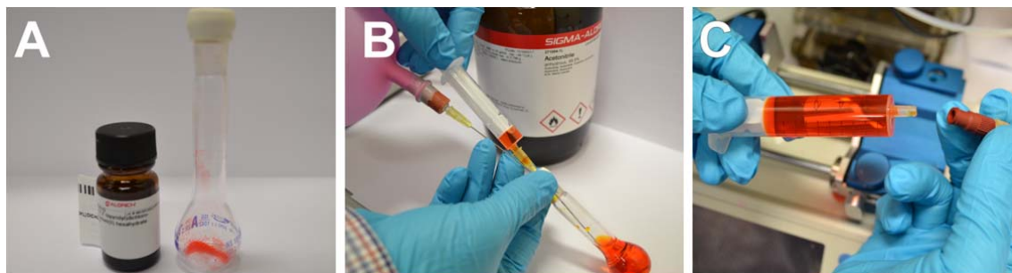
Figure 11 | Example of the preparation of a reaction solution (here, Ru(bpy) 3 Cl 2 · 6H 2 O in MeCN) (A), transferring to syringe (B) and connecting to the microfluidic system (C). Note the absence of bubbles inside the syringe.
