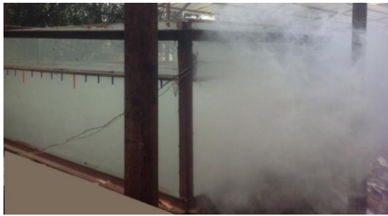
Figure 12. Smoke at exit of tunnel (60s after water system discharged)
