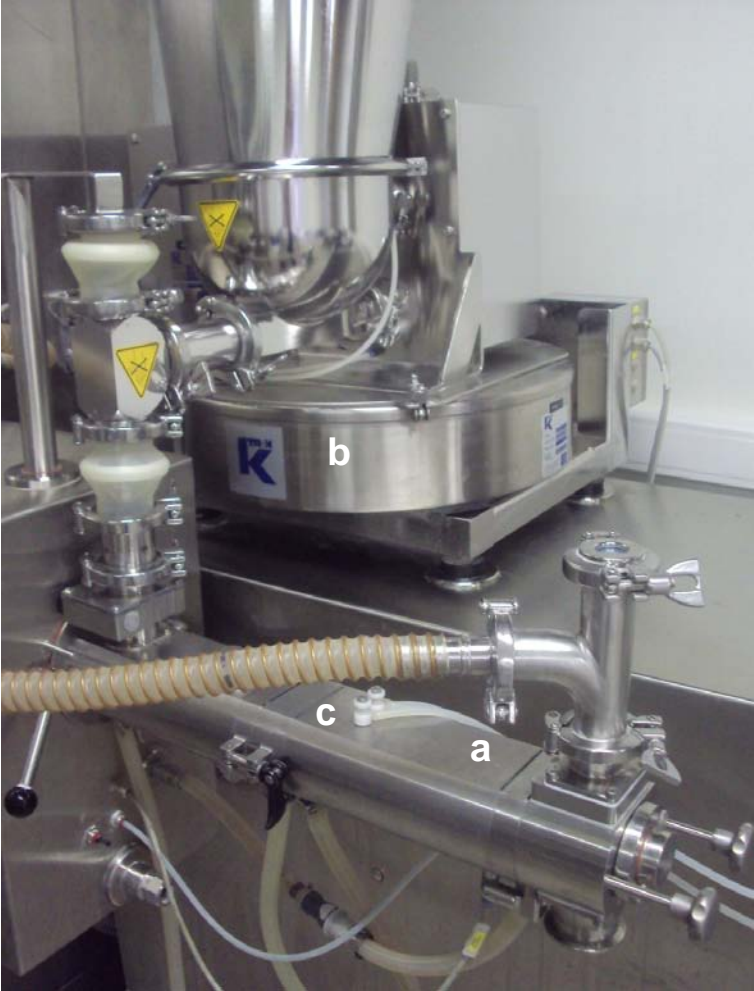
Figure 1: Consigma™-25 granulation unit: high-shear twin screw granulator (a) with K-Tron KT20 loss-in-weight feeder (b) and gravimetric liquid addition on both screws (c).
