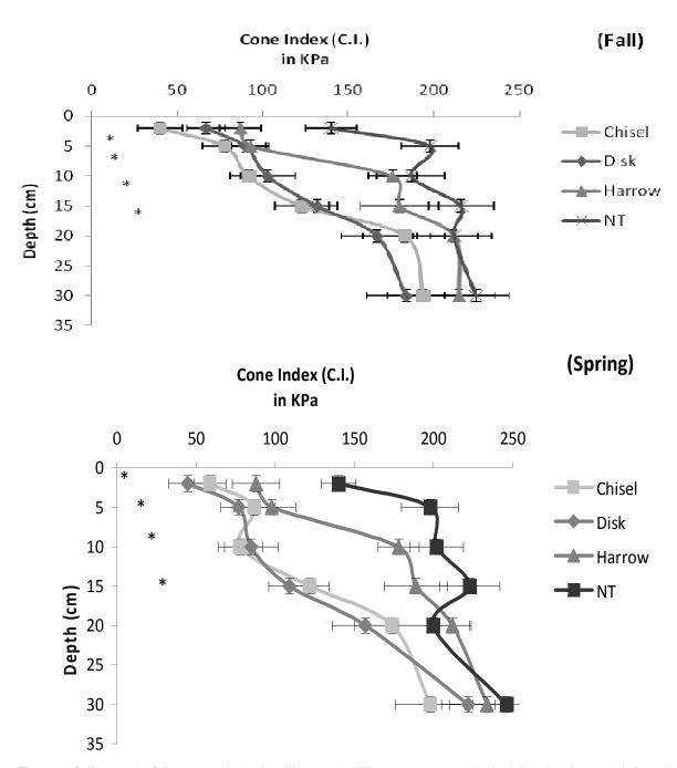
**Figure 5.** Soil strength (C.I) measured 1 h after tillage under different treatments, during fall and spring period. At each depth, (\*) means the presence of significant differences between treatments.
