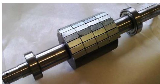
Figure 1: The rotor of the two pole machine during construction, with one magnet pole ( 7 \times 4 rectangular magnets with dimensions 20 \times 10 \times 5 mm) glued.
