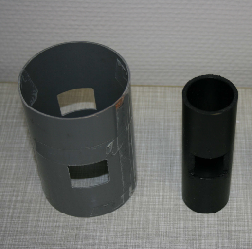
Figure 12: Cylinders used to bend the antenna: 8 cm and 4 cm diameter.
