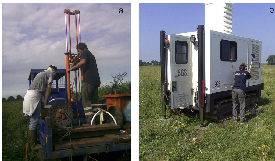
Fig. 4. (a) CPT measurements with a mobile rig on the marsh adjacent to Doelpolder Noord. (b) Seismic CPT measurements at Doelpolder Noord.
