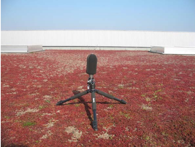
Fig. 3. Picture taken from microphone 2, positioned at low height on the green roof, towards the edge of the roof closest to the loudspeaker.
