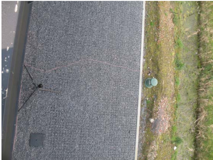
Fig. 2. Picture taken from the edge of the roof showing the reference microphone (M1) and the outdoor loudspeaker.
