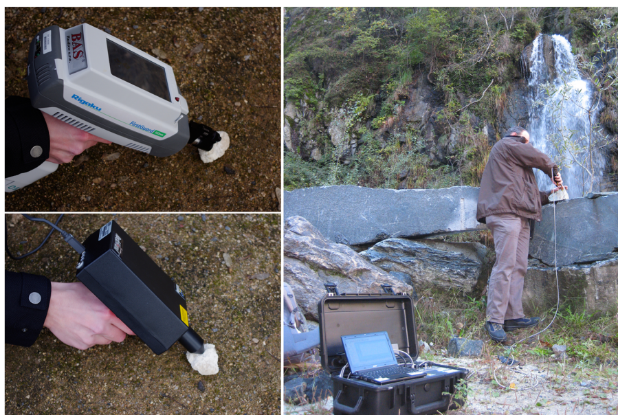
Figure 1. Handheld instruments used in this study. Upper picture 532-nm excitation diode-equipped Raman spectrometer, lower picture 785-nm excitation diode-equipped Raman spectrometer and on the right dual system (532/785-nm excitation).
