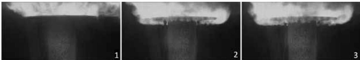
Figure 20: High speed image evidences for diffraction of blast waves during blast loading (with aluminium skin plate).
