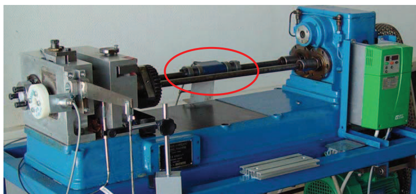
Figure 1. Modified FZG where the twin-disc tests were conducted.
