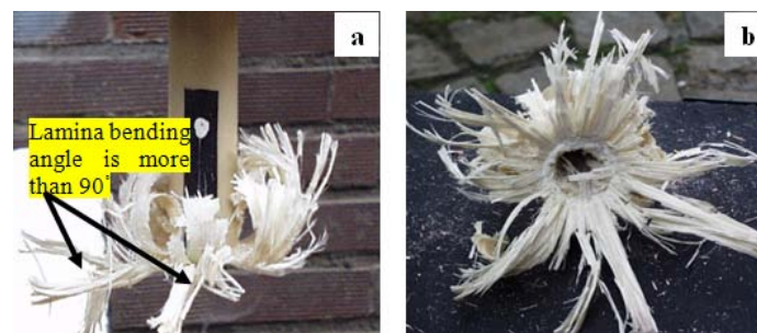
Figure 11 (a) and (b): Failure patterns of CV1 and CV2 series.
