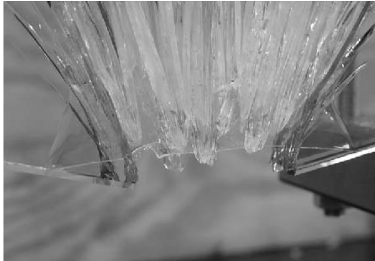
Fig. 12. Example of stretched PVB and typically large local delamination at crack origin [16]
