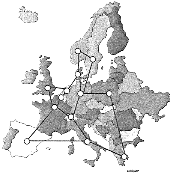
Fig. 5 Reference Grid Topology: European Core Network (13 nodes, 17 bidirectional links)
