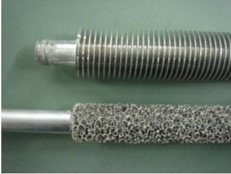
Fig. 3. A helically finned (top) as studied by Huisseune et al. [52] and metal foam covered tube (bottom).
