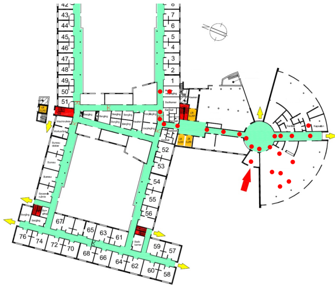
Fig. 7: The southern part of “De Vijvers” where 25 nodes were attached in the central and eastern part of the building. Their positions are marked with red dots.
