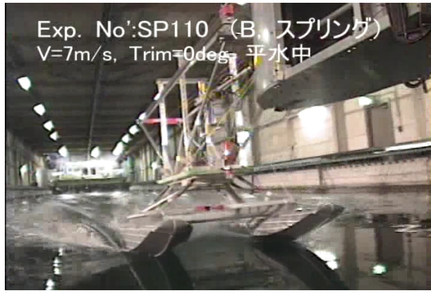
Figure 3: Experiment with the flexible support at the towing tank of Yokohama National University
