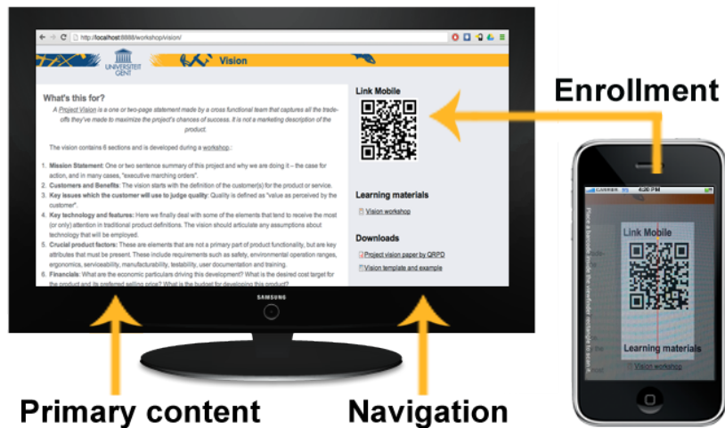
Fig. 3. Device enrollment and session synchronization via QR code scanning
