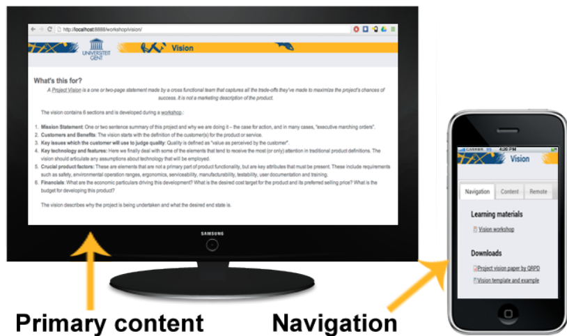
Fig. 4. Distribution of the application's presentation and navigation modules between enrolled devices
