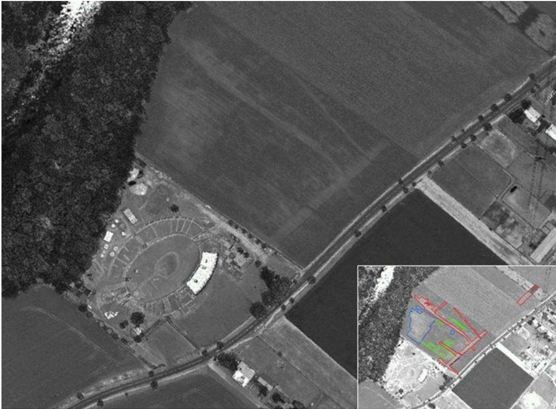
Figure 2: Detailed map of the calibrated radiometric information from ALS data (0.25 m raster size) with archaeological features; the lower right image of the same area displays an archaeological interpretation of the radiometric ALS data.
