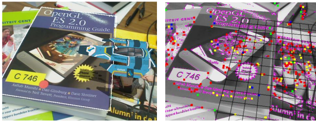
Figure 2: The augmented reality application will track feature points in the video frames (right) to enable the overlay of 3D objects (left).
