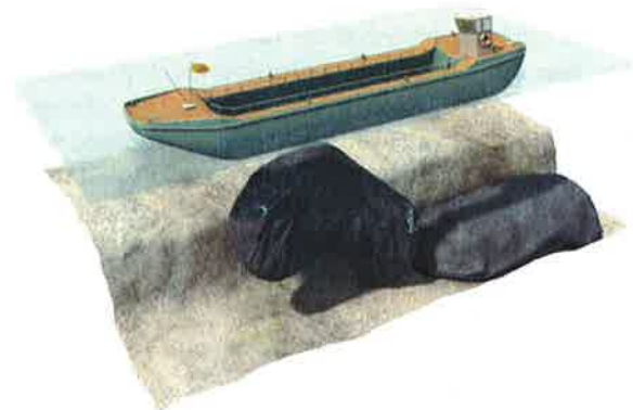
Figure 13. Artist impression dumping of a geosynthetic container
