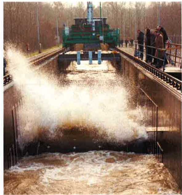
Figure 20. Wave impact on tubes during flume tests
