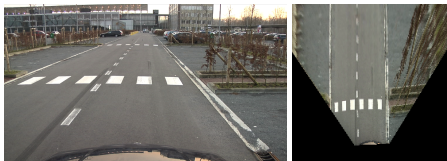
Figure 1. Example of a frame before and after perspective rectification.
