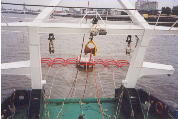
Fig. 1. Installation of the 3D seismic acquisition system on the Schelde river
