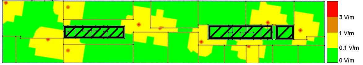
Fig. 2. Ground plan of the building that is optimized for a maximal electric field of 5 V/m at a separation of 10 cm from the AP and indication of electric-field strength (red: E > 3 V/m, orange: 3 \text{ V/m} \geq E > 1 V/m, yellow: 1 \text{ V/m} \geq E > 0.1 V/m, green: 0.1 \text{ V/m} \geq E ). The APs are located in the red/orange zones. The shaded areas indicate where no wireless coverage is required.
