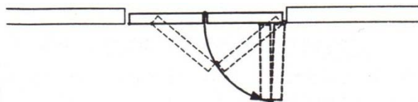
Figure 2. Kinematic principle of folding doors
