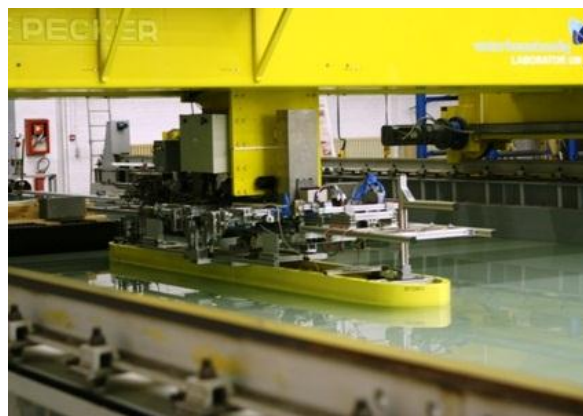
FIGURE 2 – 1/25 SCALE MODEL OF AN ECMT CLASS VA VESSEL TESTED AT THE TOWING TANK FOR MANOEUVRES IN SHALLOW WATER
