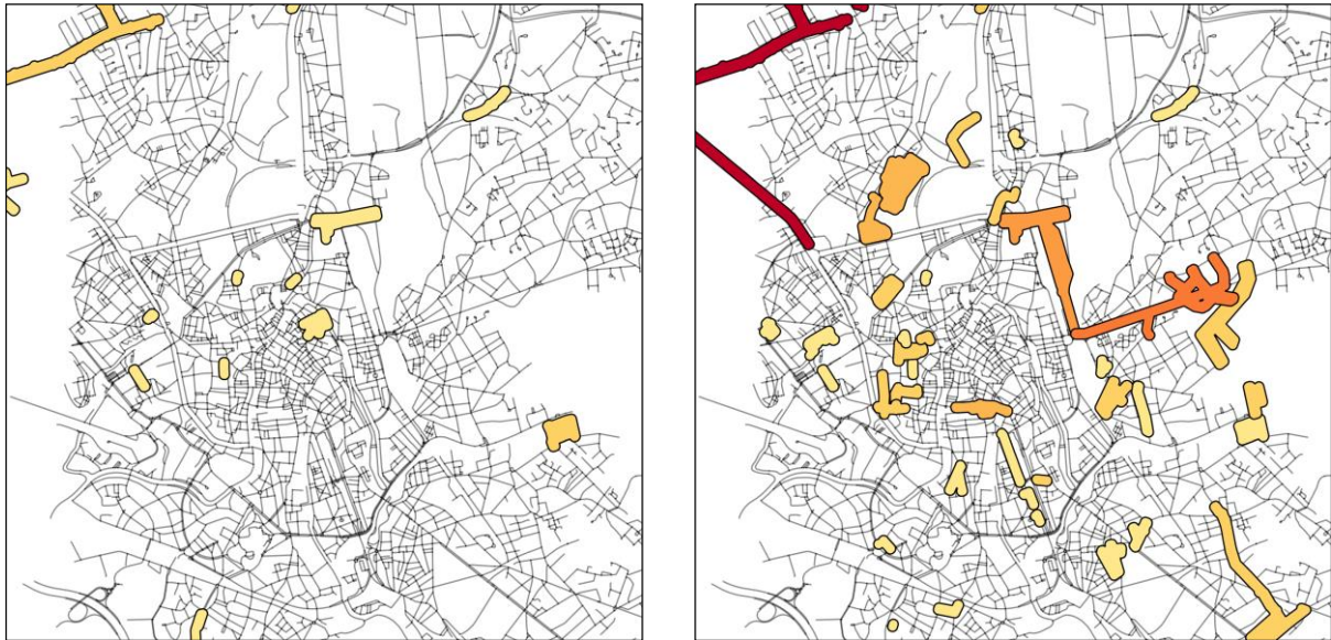
Figure 2: Optimized clustering based on geographic proximity and related deployment time has a significant impact on the amount of civil works that can be done in synergy, as shown by the difference in the amount of clustered areas and in the colour (the darker the more works within the cluster) between the initial situation (left) and the result of the optimization algorithm (right)
