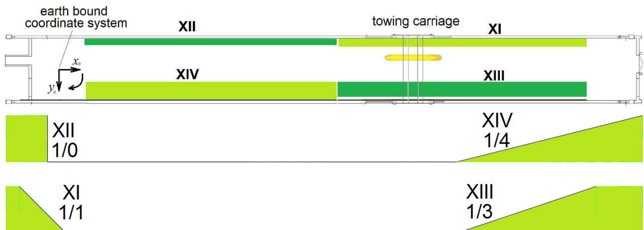
Figure 2 four different bank slopes as installed in the towing tank at FHR, plan view (top) and cross sections
