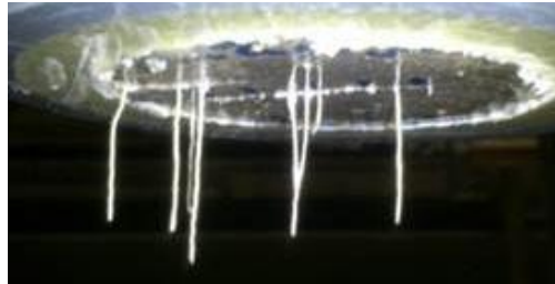
Figure 2: Stalactite formation at the bottom of the water permeability samples upon addition of 1 m% of the pH-responsive SAP.
