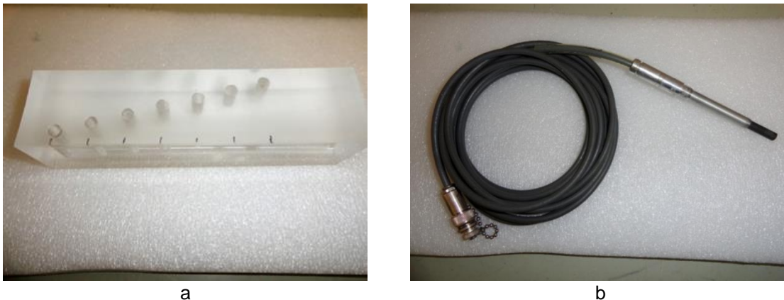
Fig. 1. Used bar of PMMA (a) and ionisation chamber (b).
