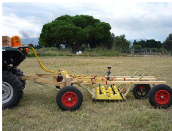
Figure 1. Three antennas fixed onto a frame towed behind an ATV, with a distance between the antenna midpoints of 0.25 m. The total station prism is mounted as lowly as possible above the center of the middle antenna, to minimize errors due to uneven topography. An odometer wheel triggers the system every 0.05 m.
