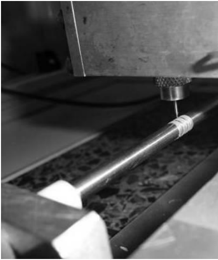
Figure 1: winding of tube scaffolds on BioScaffolder apparatus
