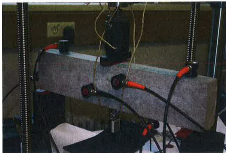
Figure 1: Acoustic emission measurements during a crack width controlled three-point bending experiment at the University of Stuttgart to test self-healing efficiency [1]
