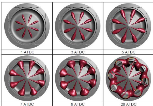
Figure 2-8: Iso-surface (Temp = 1500[°C]) for 1°-20° ATDC
