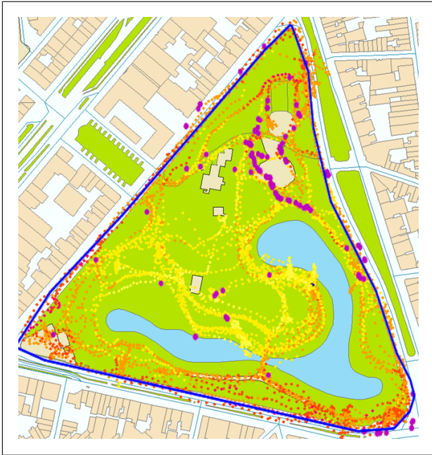
Figure 3. Map of Stadspark. The park border is shown in blue. The yellow-to-red colored dots represent the 1-minute moving average of the A-weighted sound level, sampled every 10 seconds. The purple dots indicate the activation of vocalization concept neurons in the auditory attention model.
