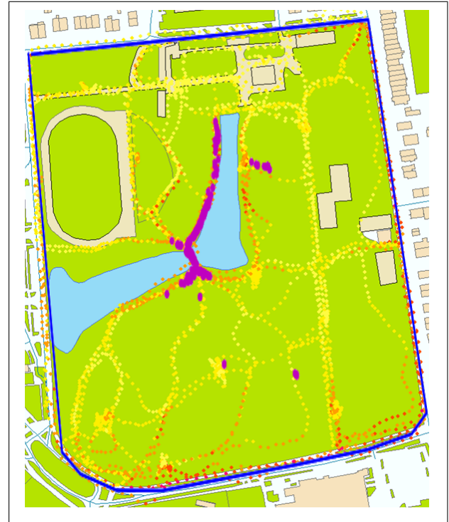
Figure 4. Map of park Sorghvliedt. The park border is shown in blue. The yellow-to-red colored dots represent the 1-minute moving average of the A-weighted sound level, sampled every 10 seconds. The purple dots indicate the activation of water sound concept neurons in the auditory attention model.
