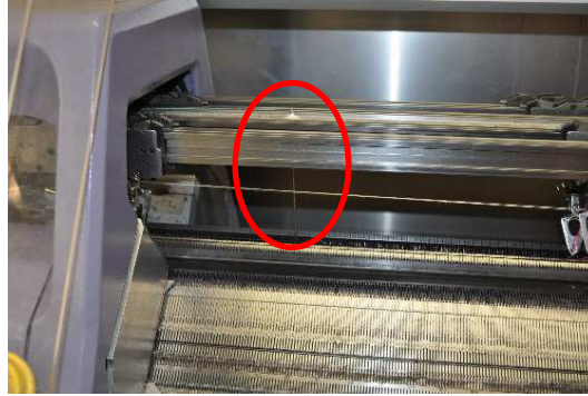
Figure 4 Supply system for bi-axial reinforcement
