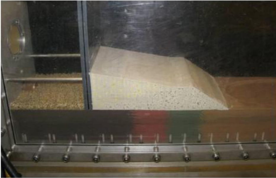
Figure 8. Dike model used for piping tests. The vertical wall was necessary to create sufficient high gradients.
