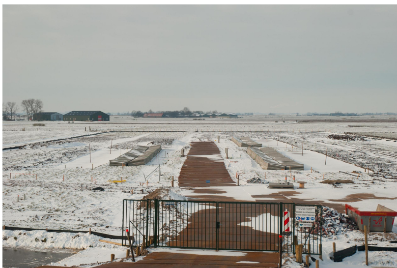
Figure 1. left: pre-loading for multistage loading tests, concrete slabs, in wintertime. right: large triaxial test.
