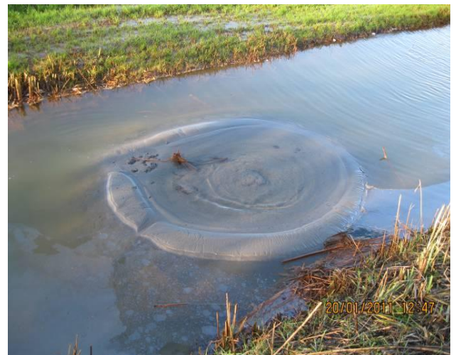
Figure 3 : Sand boil during high water period of 2011 (Hurwenen, The Netherlands)
