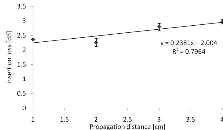
Figure 4. Measured optical loss at 850 nm, resulting from the cut-back technique. A propagation loss smaller than 0.24dB/cm was found.
