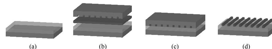
Figure 1. Process flow. (a) Spin-coated Sylgard®184 cladding; (b) LS-6943 liquid core material applied; (c) PDMS pressed between cladding and master mould and thermally cured; (d) Master mould removed.
