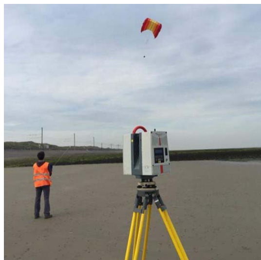
Figure 3: Image based modelling using a kite (KAP)
