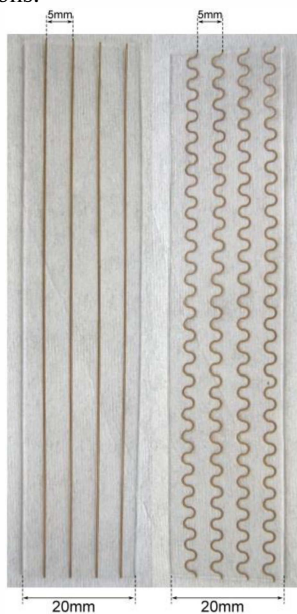
Figure 6: resulting samples (a) straight tracks (b) meandered tracks
