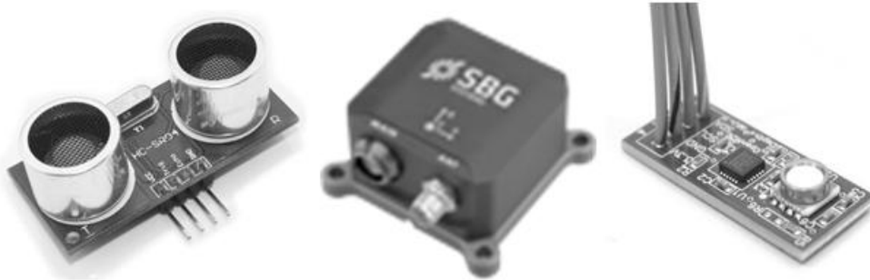
Figure 3: Ultrasonic distance meter for use in combination with a microcontroller (left, source: http://arduino.cc ), integrated INS / GNSS system (centre, www.sbg-systems.com ) and integrated IMU, compass and depth sensor (right, source: www.openrov.com )
