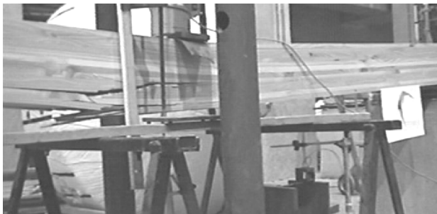
Figure 6 Destructive bending test of the Douglas-resorcinol composite
