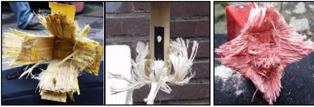
Figure 4 Failure patterns of tubes from experimental test.
