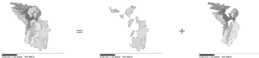
Fig.2: The separation of a partially transformed grain into an austenitic (middle) and a martensitic part (right)
