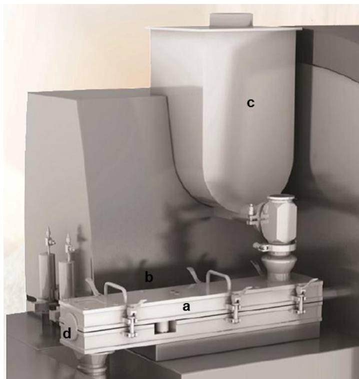
Figure 1. ConsiGma™-1 system with (a) high-shear granulator barrel, (b) liquid addition on both screws, (c) gravimetric feeder and (d) granulator exit to be optionally coupled to a fluid bed dryer.
