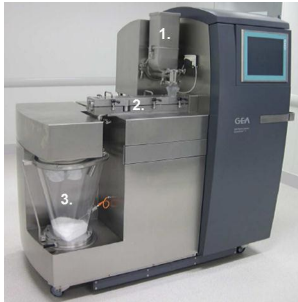
Figure 16. ConsiGma™-1 with: 1. Powder dosing, 2. Granulator barrel, 3. Fluid bed dryer [courtesy GEA Pharma Systems].
