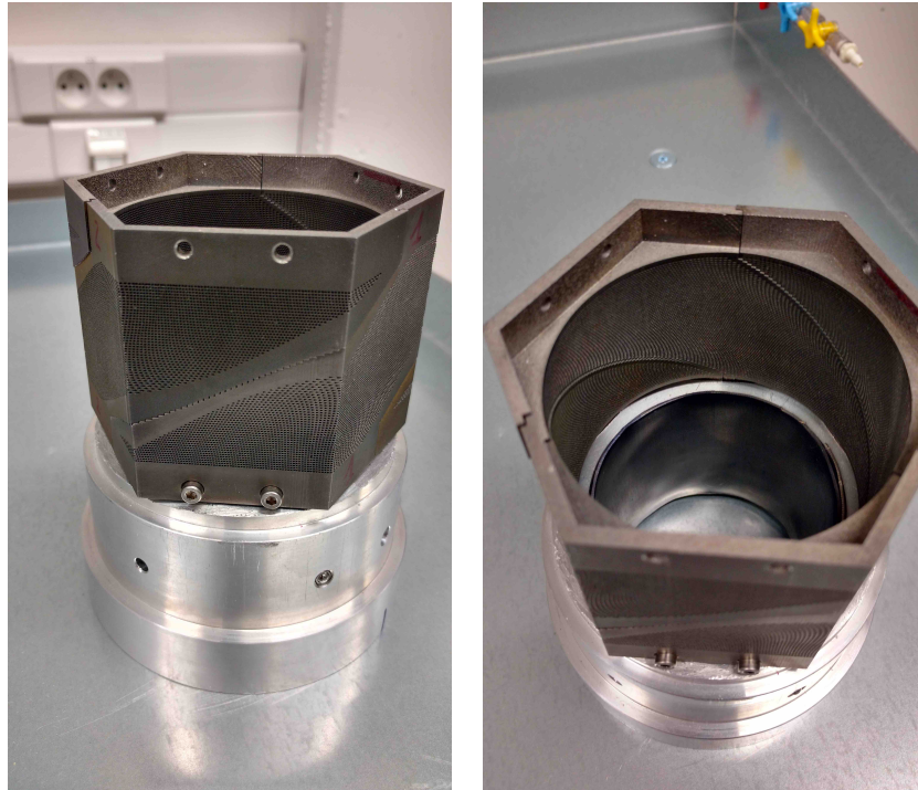
Figure 7.11: Photos of the full collimator from two different views, showing the three printed parts fitted together.
