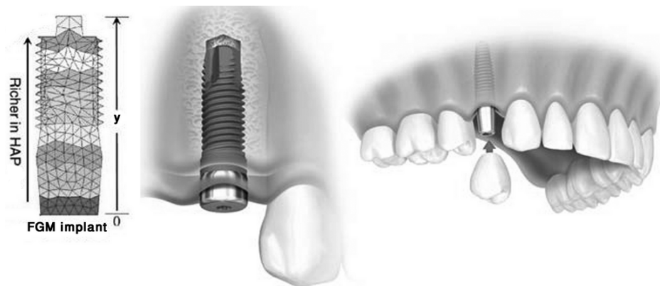
Figure 1.8. Schematic view of FGM dental implant with graded material composition.
